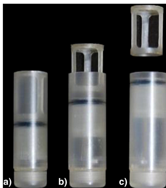
Fig. 4. Spring loaded capsule releasing drug reservoir [9].
